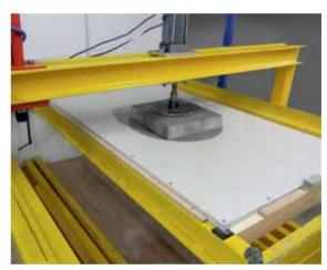
Tests have shown that the Impey Aqua-Dec EasyFit will easily support over 300kg (47 stone) without the need for under boarding
